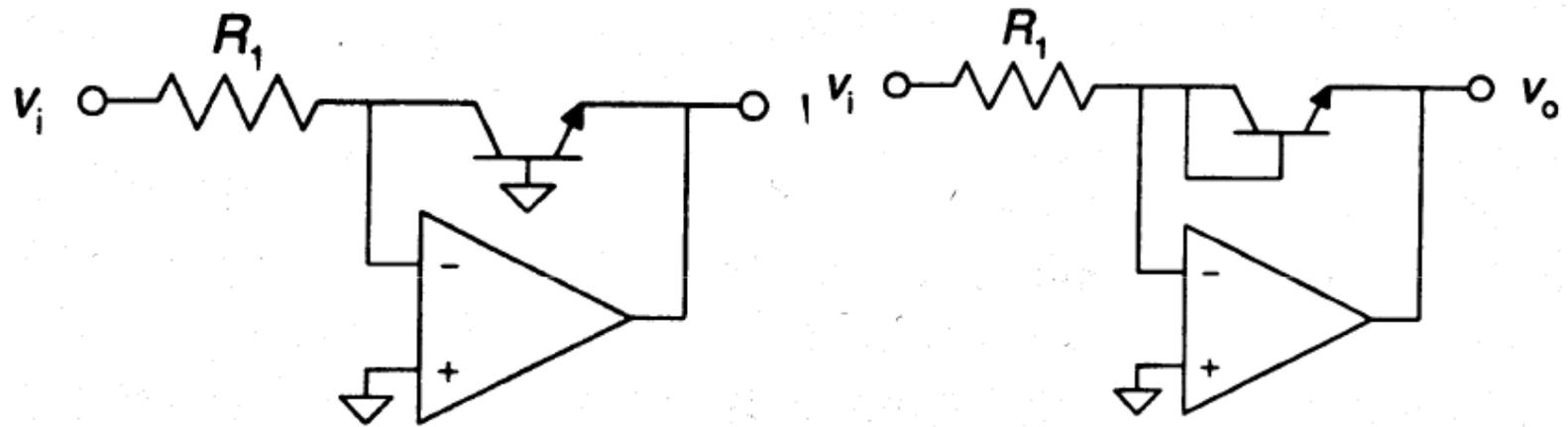
Fig: Transdiode Log Amplifier
