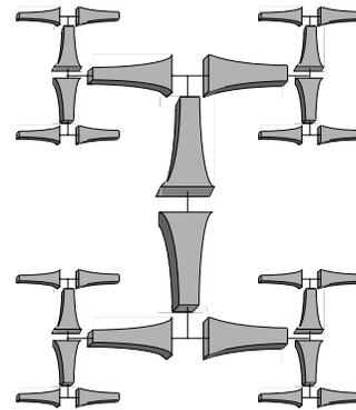
Figure 1: Exponentially tapered H-tree
