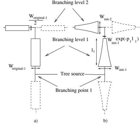
Figure 3: Interconnect in an H-tree a) uniform tapering b) exponential tapering
