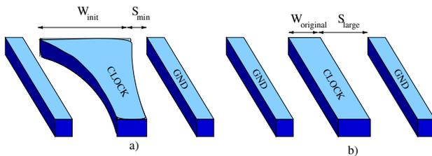
Figure 4: Coplanar clock line a) exponential tapering b) uniform line with wider spacing
