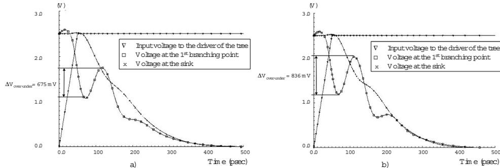
Figure 5: Waveforms at different nodes within the tree a) exponential tapering b) uniform tapering (with large spacing)
