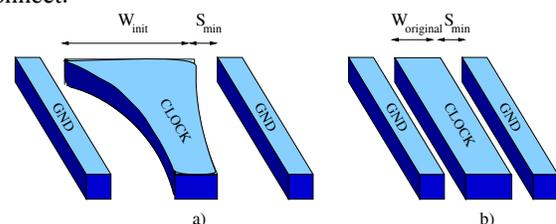
Figure 2: Coplanar clock line a) exponential tapering b) uniform (no tapering)
