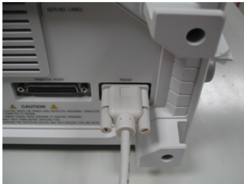
DB9 to DB9 wiring
