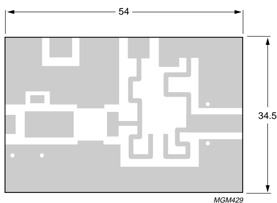
Fig.13 Printed-circuit board BLW32.
