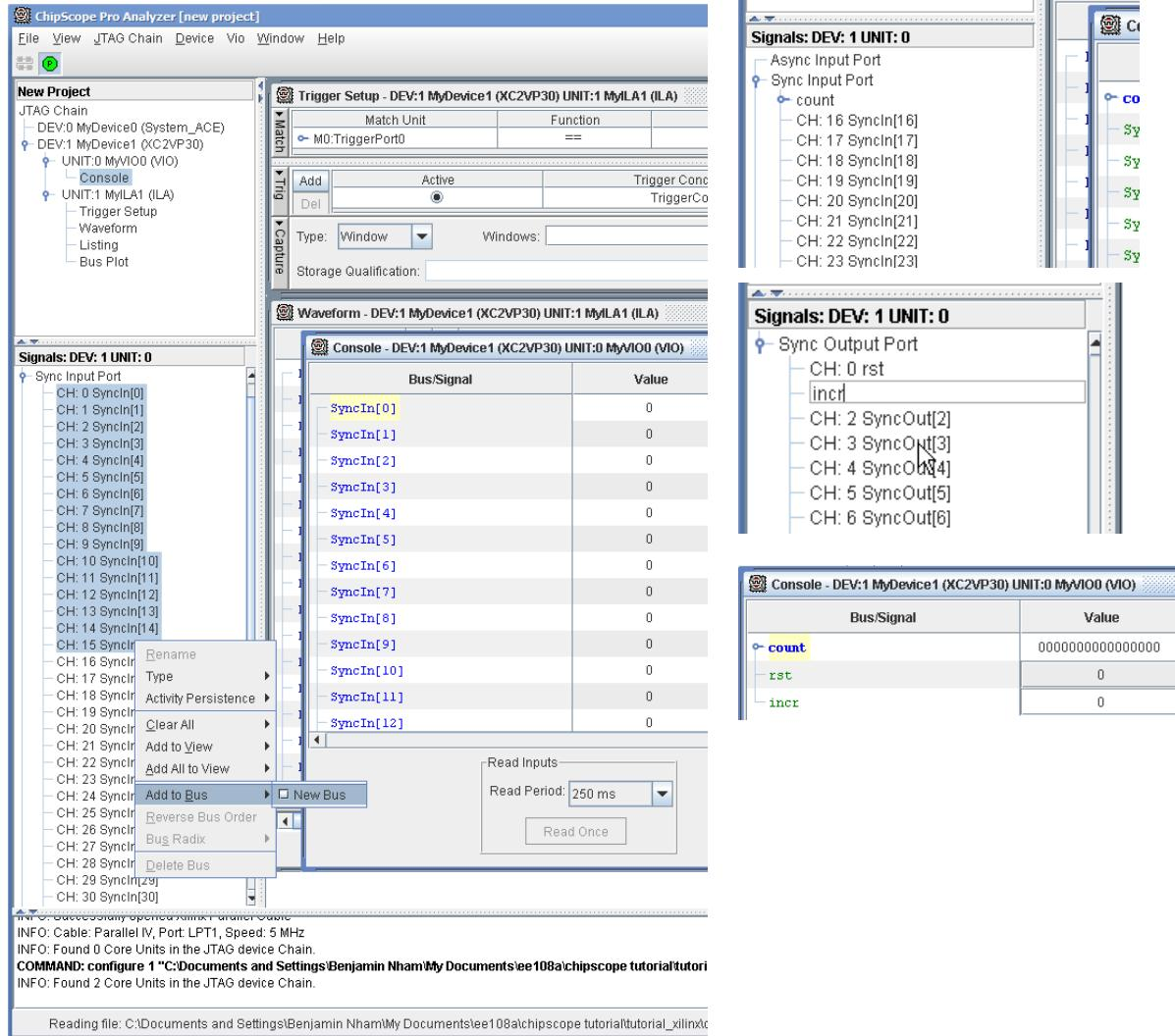
Now, onto the logic analyzer. Double click on the ILA unit in the top-left hand corner of ChipScope Analyzer to bring up the Waveform and Trigger windows. For the waveform, you'll want to do the same thing as we did above—rename the signals so they mean something useful. Select the 0<sup>th</sup> bit of the data port and rename it reset. Select the 1<sup>st</sup> bit of the data port and rename it incr. Select bits 3-18, add them to a bus, and rename the bus count.
