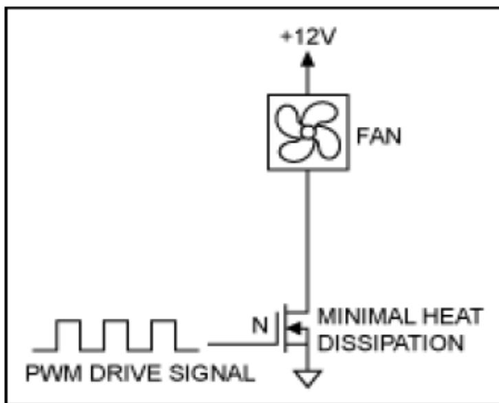
Here i am using IRF540N MOSFET, SAN ACE 12V DC Fan, I am applying 5V PWM signal to the IRF540N MOSFET.
