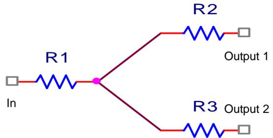
Figure 3: Layout of a 2 way power divider
