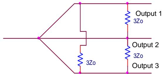
Figure 4: Layout of a 3-Way power divider
