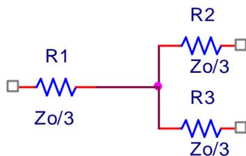
Figure 2: Layout of 2-Way resistive divider
