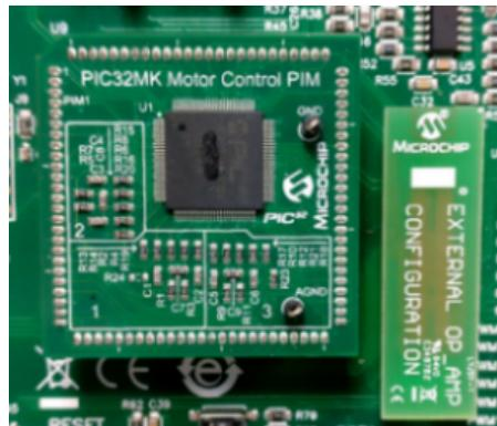
5. Connect the programmer and debugger using the J11 connector.
