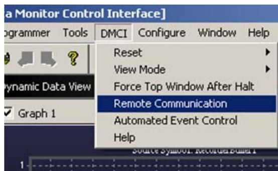
11. Remote Communication needs to be established, as indicated in the following figure (the communication baud rate should be set to 38400, while the COM port used depends on your particular settings).
