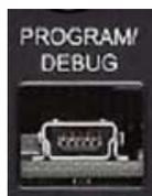
7. For enhanced demonstration, the application requires the Real-Time Data Monitor (RTDM). Users can connect a mini-USB cable from their computer to the J6 connector of the dsPICDEM MCHV Development Board.
