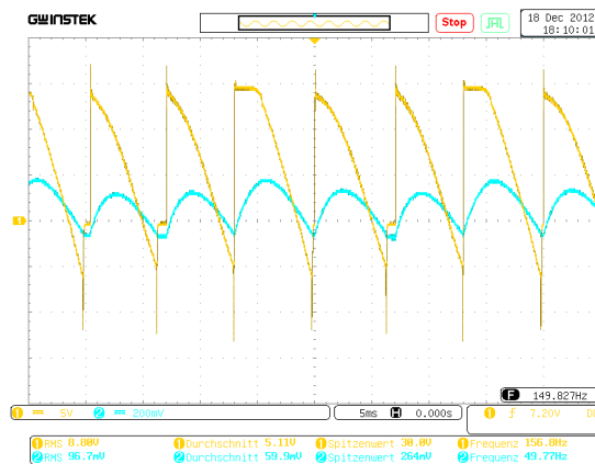
pic. 3.5.1.3 triggering angle \alpha = 90^\circ
