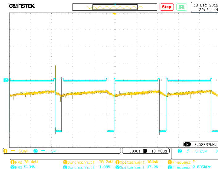
pic. 5.4.1.3.4 duty cycle g = 0,4 and f_D = 1 \text{ kHz}
