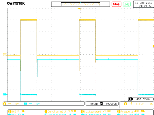
pic. 5.4.1.1.8 control voltage U_S = -5 V
