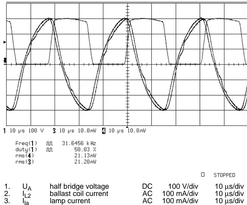
Fig.11 Lamp current and Ballast Coil Current, CFL18W circuit
