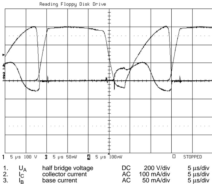
Fig.9 Switch Behaviour of TR2, CFL18W circuit
