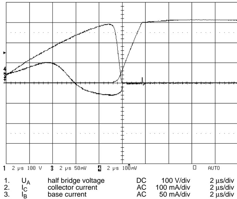
Fig.7 Switch-off Behaviour of TR2, CFL10W circuit
