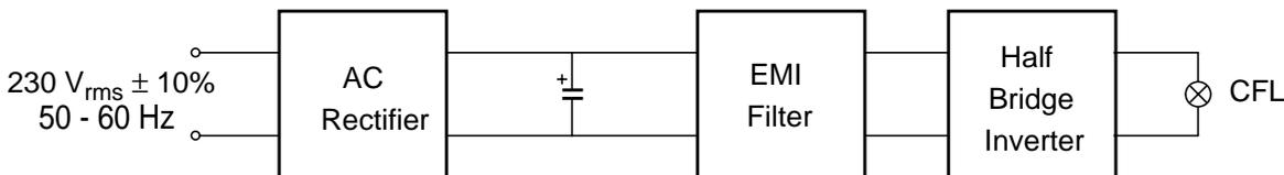
Fig.1 Block Diagram CFL circuit
