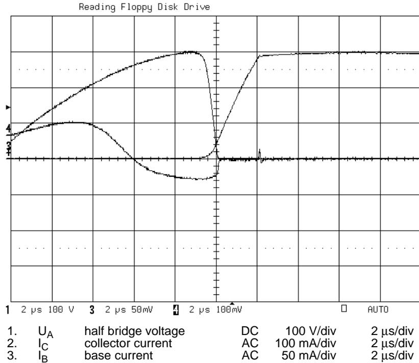
Fig.10 Switch-off Behaviour of TR2, CFL18W circuit
