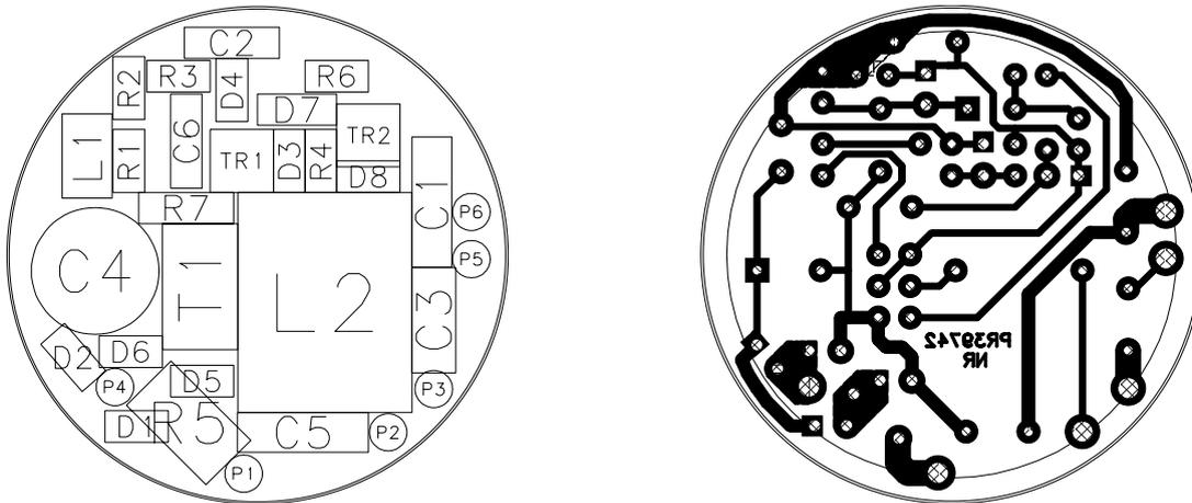
**Fig.5 Component- and Copper Side of PR39742**
