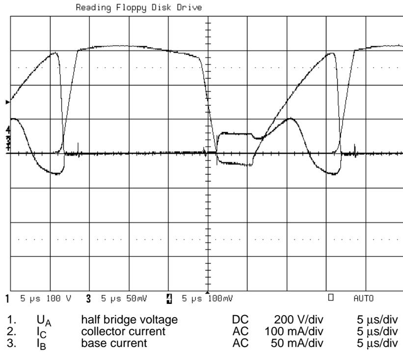
Fig.6 Switch Behaviour of TR2, CFL10W circuit
