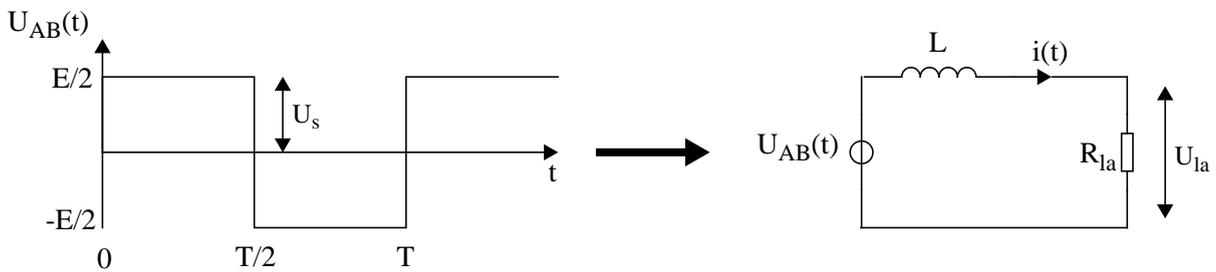
Fig.12 Equivalent Load Circuit.
