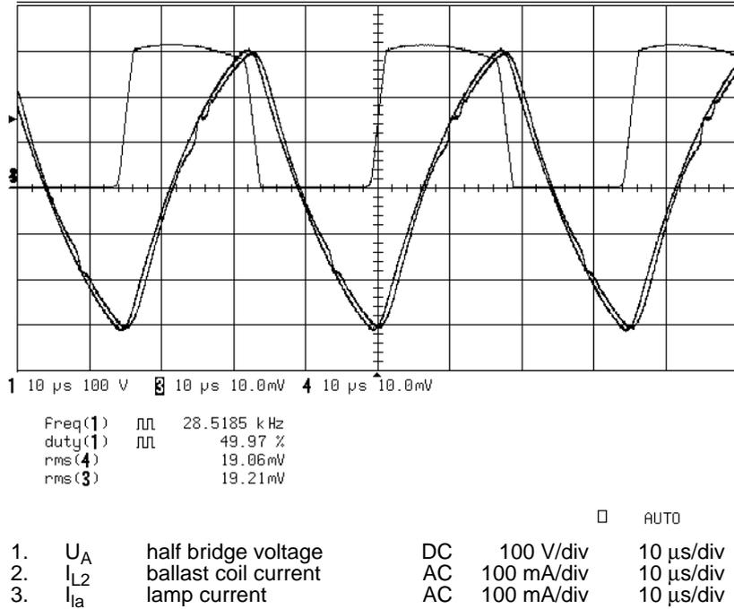
Fig.8 Lamp current and Ballast Coil Current, CFL10W circuit
